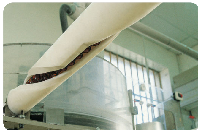
360° turning unit with straight central section
