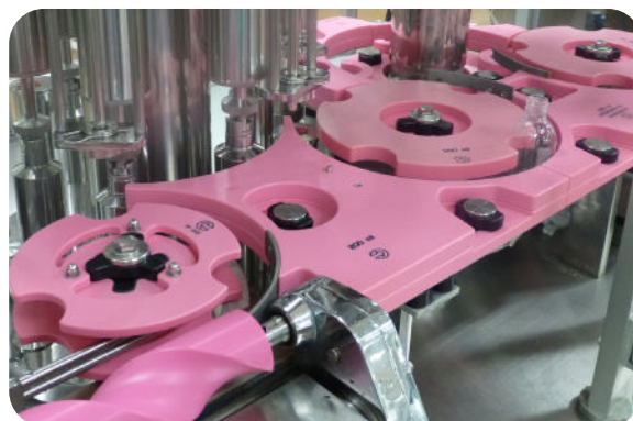
Rotobloc : Quick-change format system adaptable to any type of machine.
