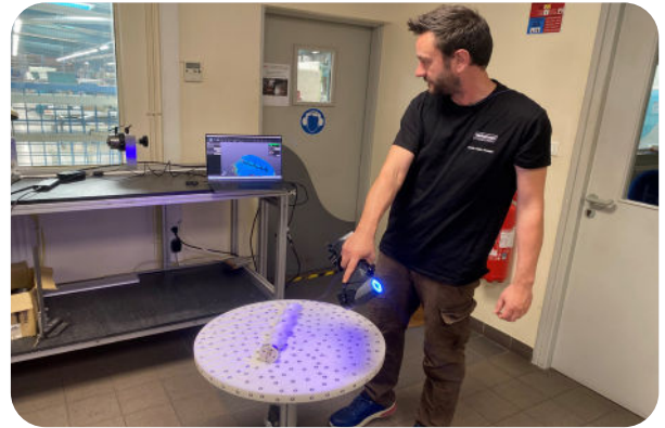
Scanning of parts and machine bases with a 3D scanner
