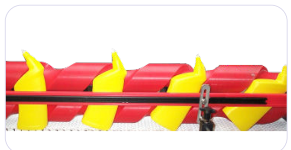
Tilting: filling of inclined bottles
