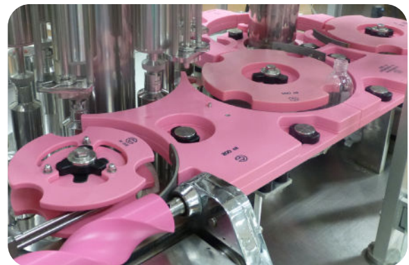
Rotobloc : Quick-change format system adaptable to any type of machine.
